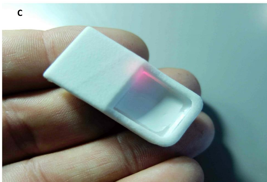
Figure 2.5.2.2 Assembled implant. (A-B) Front and back view of PA 2200 3D printed implant encasings and cell compartment, with RFID chip, LED and cellulase sensor inserted (marked with arrows). (C) Implant activated on field generator to emit NIR light, held approximately 2 cm from the surface of the generator plate.
